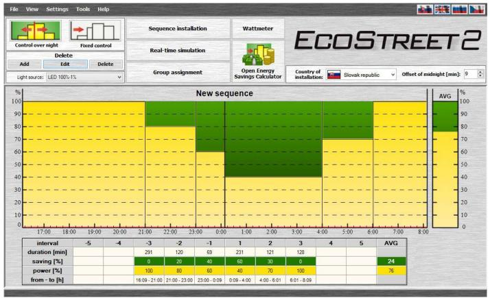
The programming software Ecostreet 2 enables creating sequences, which are then installed into DIM BAR devices by using the powerline master Ecobox 2 connected to a PC. It also features an energy savings calculator for predicting savings for a selected period with a display of sunrise and sunset according to an integrated calendar. The sequence can contain up to 10 intensity changes in the range of 0 – 100%.
